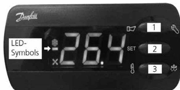
Fig. 2: Danfoss controller – controls and displays (symbols)
